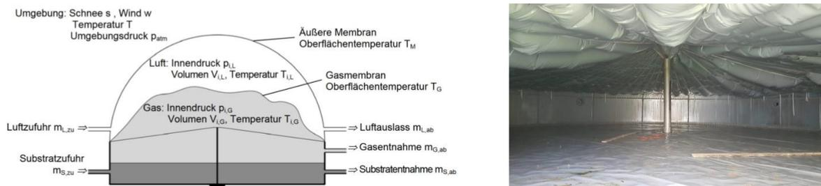
Figure 1: Schematic sketch of a biogas storage system (left), No gas pressure in the biogas-silo, gas membrane lies on the belts (right)
