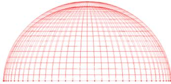
Figure 6: Double Chamber with warp- and weft directions of the textile fabric
