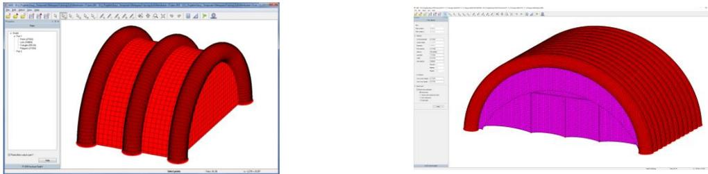
Figure 3: Pneumatic tube systems combined with mechanically stressed membranes
