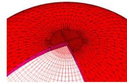
Figure 7: 2 chambers are described by triangular surface elements
