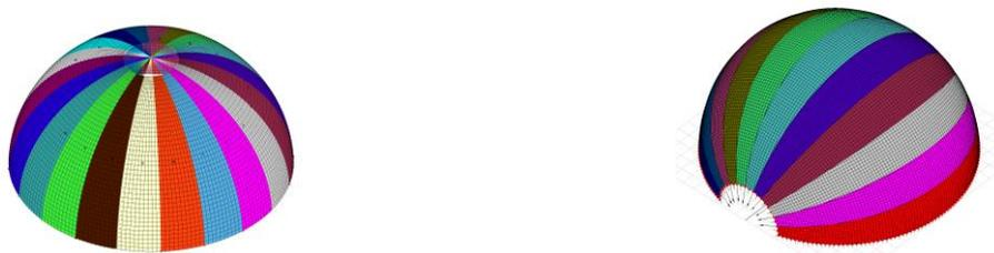
Figure 5: Radial (left) and parallel (right) cutting patterns
