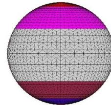
Figure 10: Wind load zone under 3 different wind directions (0°, 45° and 90°).
