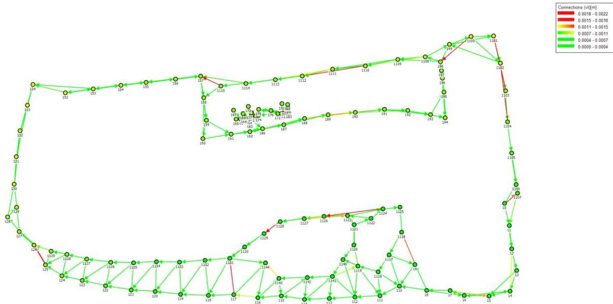
Figure 2: Colour residuals in the Network Analyser (data courtesy of BIMm Services GmbH)
