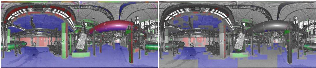
Figure 10: Detected planes in a scene (left) and used planes within a registration (right)
