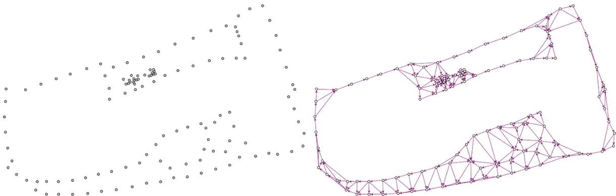
Figure 3: Pre-oriented scans as imported (left) and triangulated network (right)
