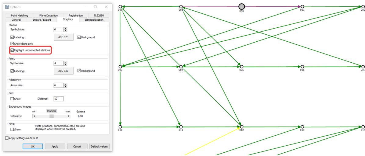
Figure 8: Highlighting unconnected stations within a network
