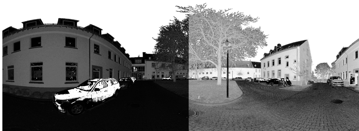
Figure 4: Generated intensity image before (left) and after (right) histogram equalisation (Data courtesy of intermetric GmbH)
