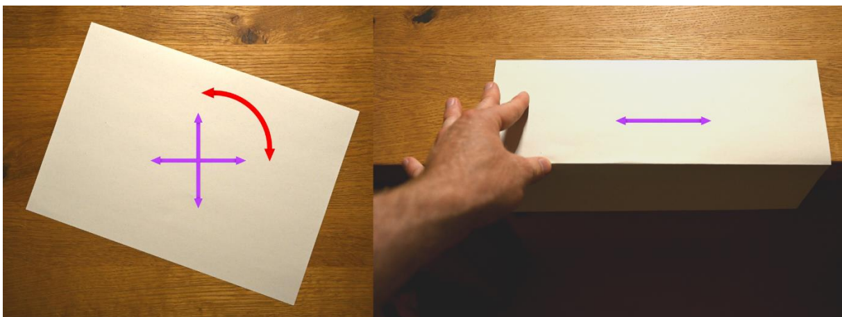
Figure 2: Overlap between two datasets that allows you to solve 3 (left) respectively 5 degrees of freedom (right)
