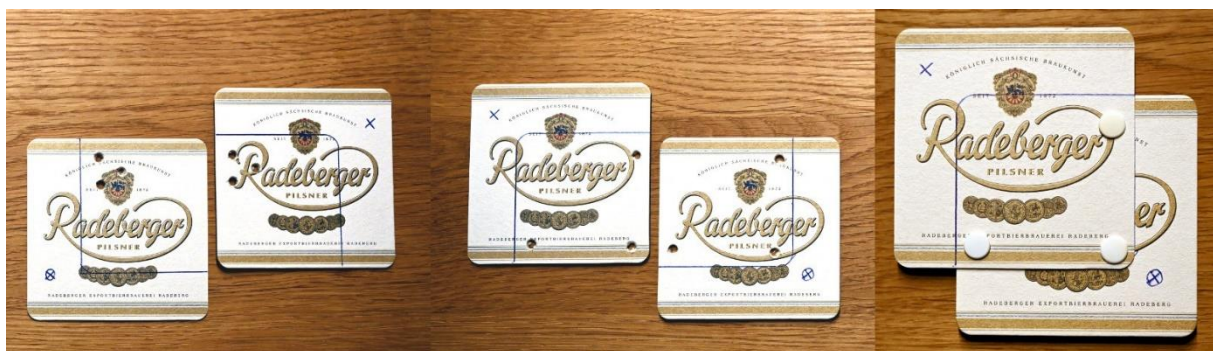
Figure 2: Two scans with a poor distribution of artificial targets (left), covering the Gruber region (centre) and finally “registered” by thumbtacks (right)
