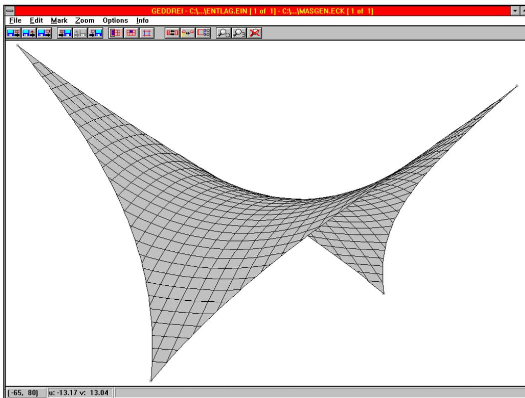
Figure 7: Simple saddle surface.
