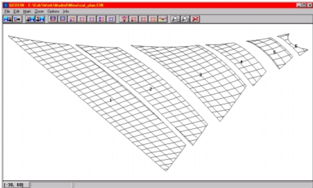
Figure 11: Individual doubly-curved half cloth strips cut from form-found surface.
