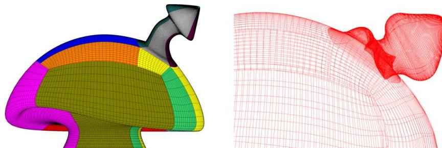
Figure 13: Detailed views: Geometrically defined shape (left), statically calculated shape under internal pressure (right)
