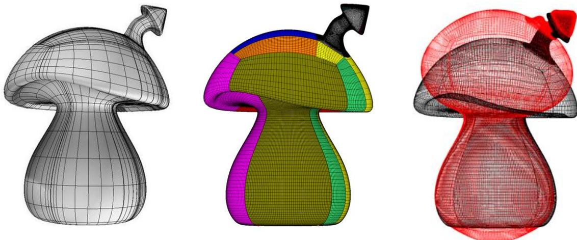
Figure 12: Geometrically defined model (left), discrete model (middle), comparison of the geometrically defined shape (black) with the shape statically calculated under internal pressure (red) (right).
