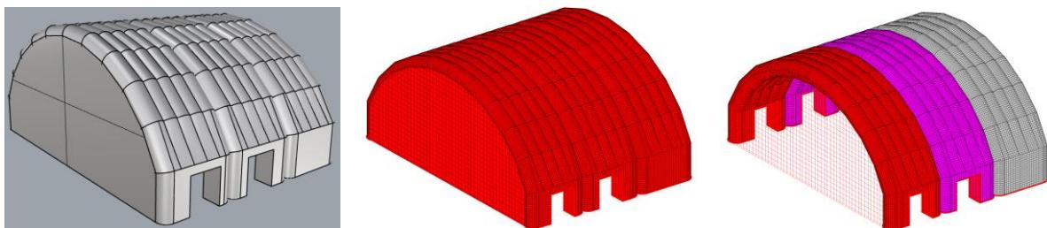
Figure 3: Combined pneumatically and mechanically stressed structure with nurbs (left), discrete overall system (middle), visualisation of the 3 chambers in the discrete model (right)
