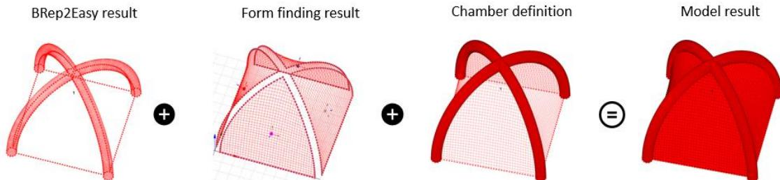
Figure 11: Sequence of the modelling with combined mechanical and pneumatic stressed structures
