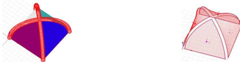
Figure 10: Force density form-finding based on boundaries from CAD
