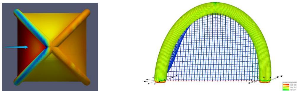
Figure 15: Wind pressures from the digital wind tunnel (left), stresses, reaction forces and deformation (right)
