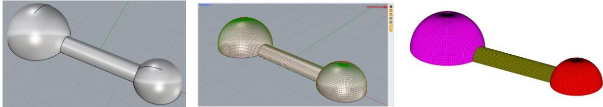
Figure 7: Combination of pneumatically feasible elements by intersecting of nurbs surfaces (left), Brep-object and overlayed discrete model (middle), discrete model (right)
