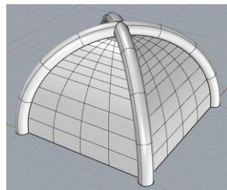
Figure 8: 2 intersecting air pipes and 4 mechanically stressed walls
