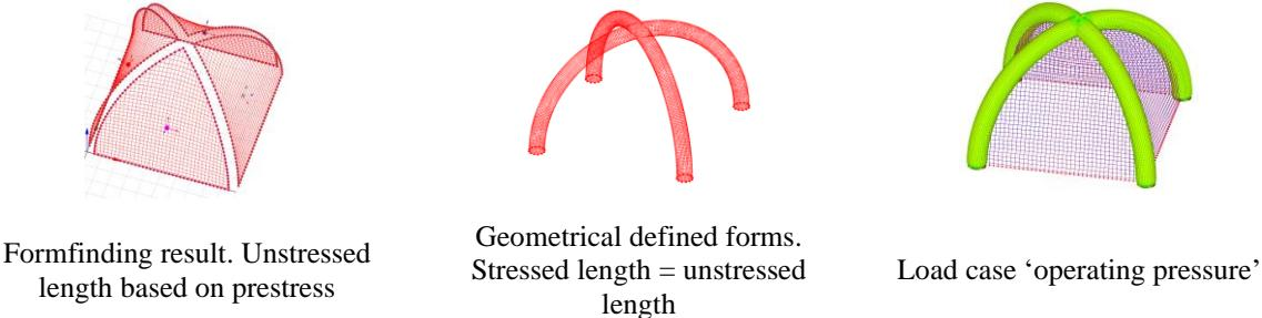
Figure 14: Combination and calculation of the ‘operating pressure’ load case
