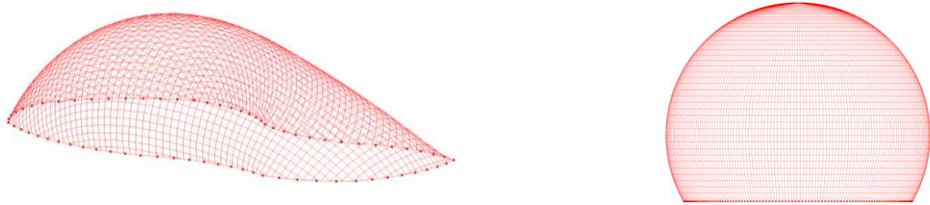
Figure 1: Pneumatic structure over an arbitrary boundary (left), pneumatically feasible structures (right)
