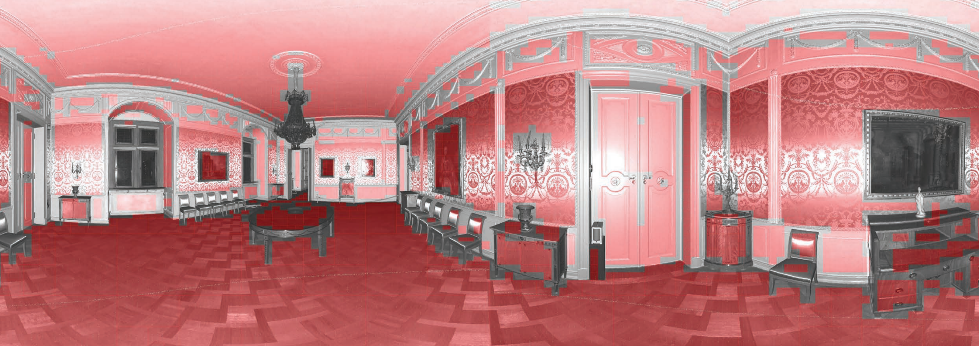
Detected planes in a scan of an electoral living room (colored planes) Source: FPK
