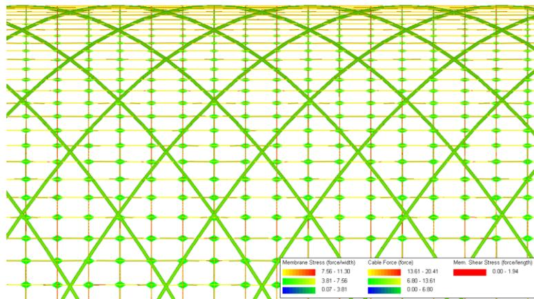
Figure 5: Constriction of the membrane by cables
