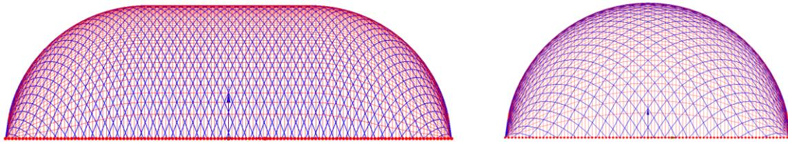
Figure 4: Big gas holder with equidistant cable mesh
