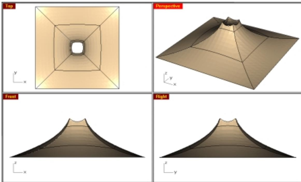
Figure 10: 8x8 production surface showing the new seam layout.
