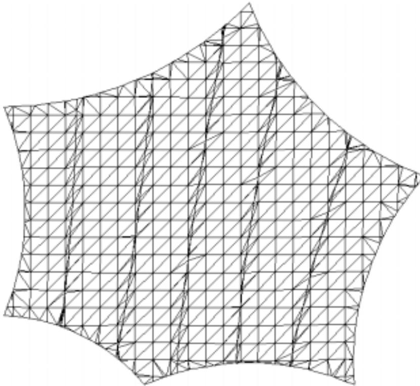
Figure 6: Geodesic lines splitting a discrete membrane surface into strips.
