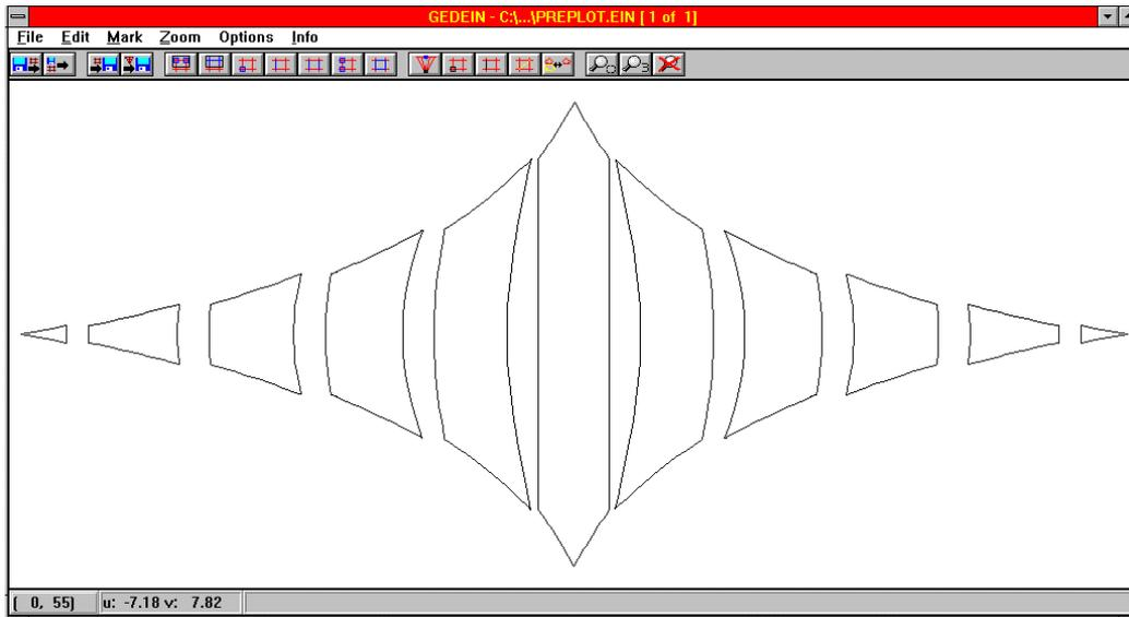
Figure 8: Vertical planar cut patterning of saddle shown in Fig. 7.
