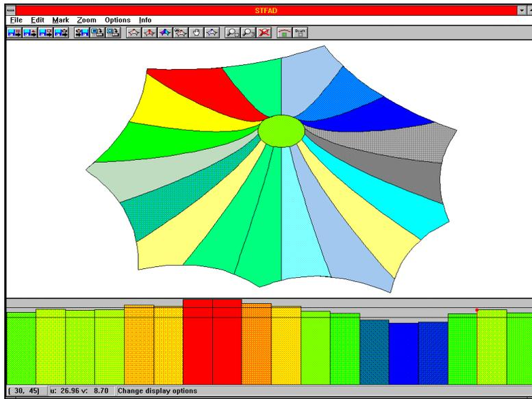
Figure 2: Easy system cutting pattern layout for the high point surface shown in Fig. 1 with graph of cloth widths.
