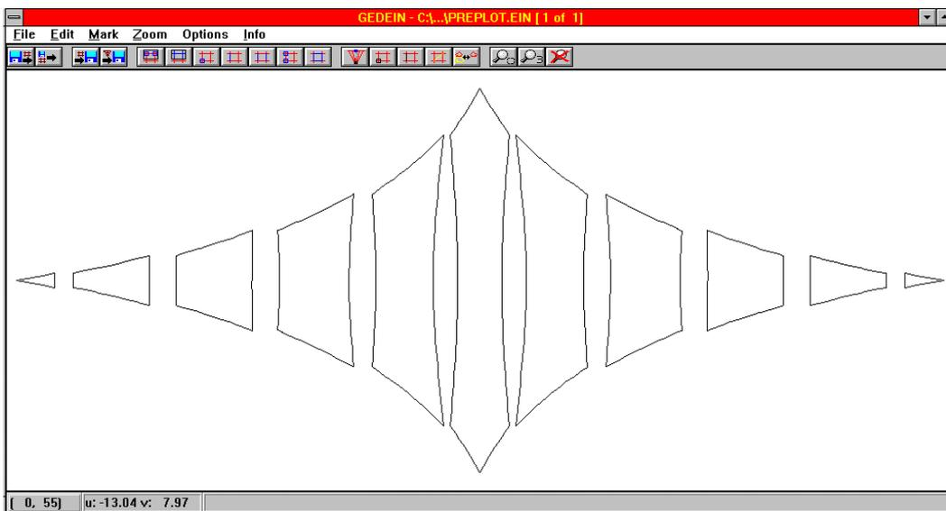
Figure 9: Geodesic patterning of saddle shown in Fig. 7.
