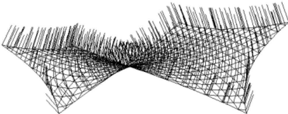
Figure 5: Normal vectors, a prerequisite for describing the curvature of the surface.
