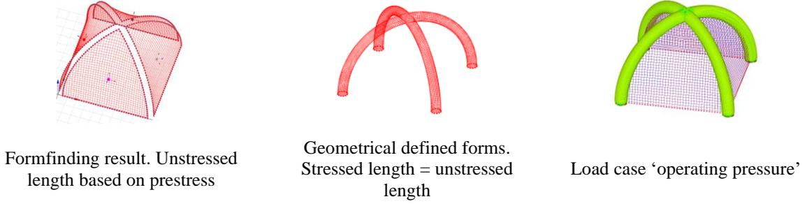
Figure 14: Combination and calculation of the 'operating pressure' load case
