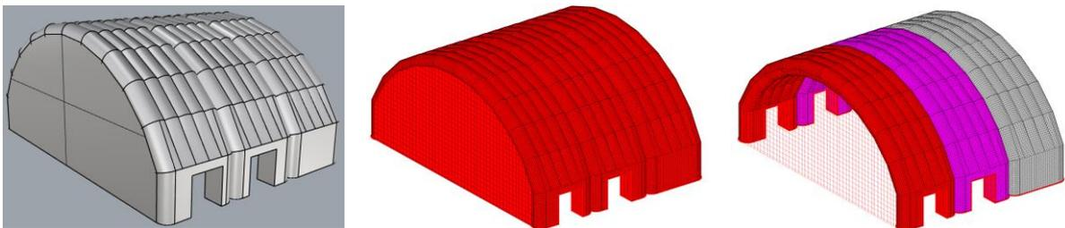
Figure 3: Combined pneumatically and mechanically stressed structure with nurbs (left), discrete overall system (middle), visualisation of the 3 chambers in the discrete model (right)
