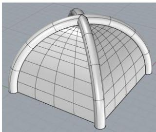
Figure 8: 2 intersecting air pipes and 4 mechanically stressed walls
