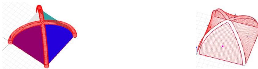
Figure 10: Force density form-finding based on boundaries from CAD
