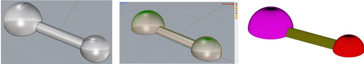
Figure 7: Combination of pneumatically feasible elements by intersecting of nurbs surfaces (left), Brep-object and overlaid discrete model (middle), discrete model (right)
