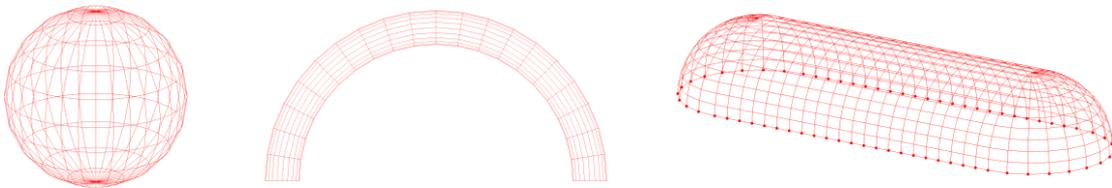
Figure 6: Discrete sphere and tube model (left), 2 quarter spheres and 1 half cylinder combined to a discrete model (right)
