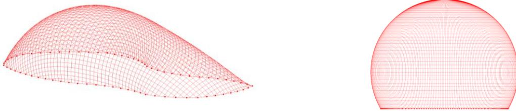
Figure 1: Pneumatic structure over an arbitrary boundary (left), pneumatically feasible structures (right)
