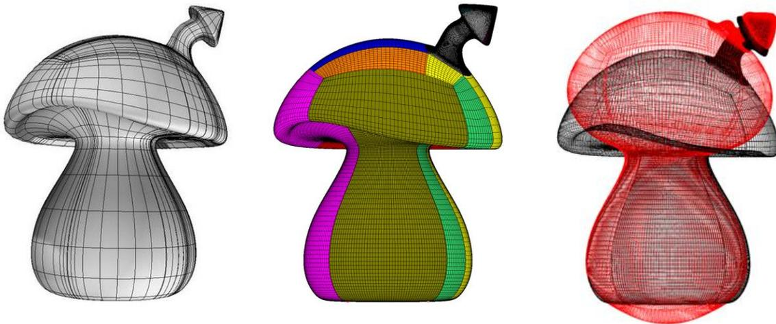
Figure 12: Geometrically defined model (left), discrete model (middle), comparison of the geometrically defined shape (black) with the shape statically calculated under internal pressure (red) (right).
