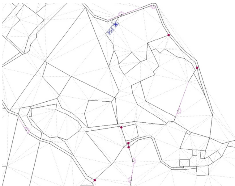
Figure 3: All vertexes of cadastral index map (including identical points, red dots) are included in Delaunay triangulation (dashed lines). The geometrical constraints (rectangularity, straight lines) are also considered.
